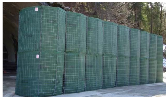
Figure 2: Example wall: Double stacked, MIL 8 Hesco Bastion wall unit used in test series 2015 / 2016
