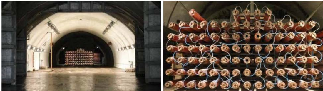
Figure 1: LBS Shock tube systems with typical gas bottle arrangement
