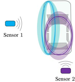
Fig. 1: Estimates of a vehicle from two sensors 1 and 2 as a light blue and a purple ellipse. Both estimates possess different uncertainties in the semi-axes and orientation represented by the more transparent versions of the estimates.
