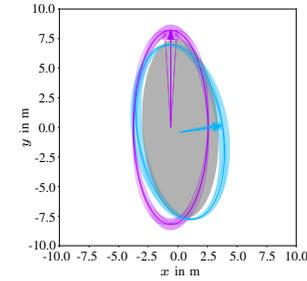
Fig. 4: Exemplary input with ground truth in gray, sensor 1 in magenta, and sensor 2 in cyan. The ellipses' respective orientation is represented by an arrow and the uncertainties are visualized as pale ellipses. Note how the measurements possess different uncertainties for the semi-axis.
