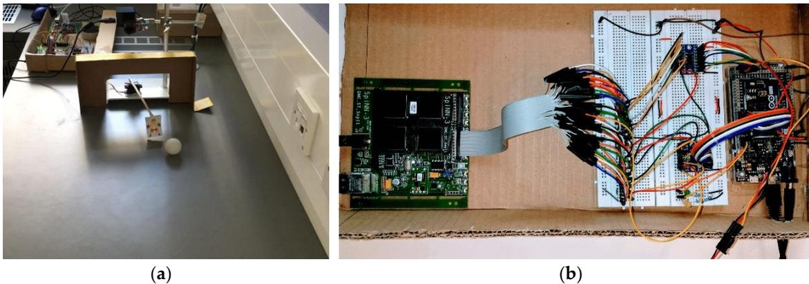
**Figure 7.** (a) Setup of the neuromorphic robotic goalkeeper. (b) Connections between the modules. One input/output port is used on SpiNNaker (SpiNN-3) board (shown left) and set in SpiNNakerLink class. Two chips on the protoboard are level shifters (1.8V to/from 3.3V), which are used between the microcontroller and SpiNNaker. The microcontroller (Arduino Due) is at the right end of the picture.
