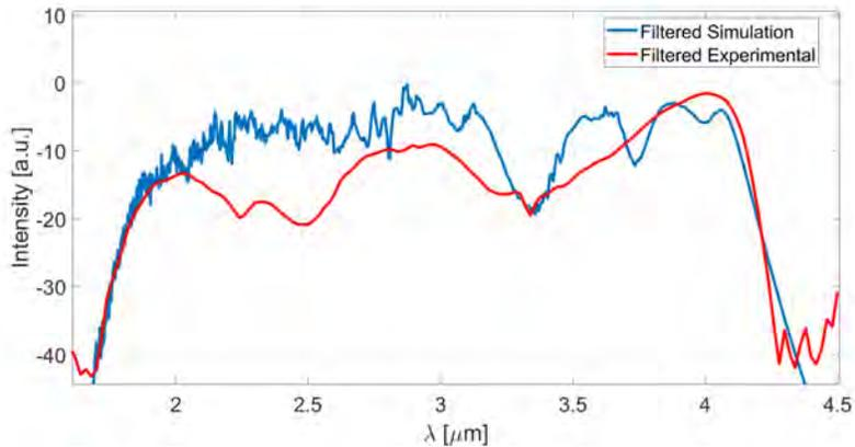
Figure 7: Filtered spectrum injected in the chalcogenide fiber.
