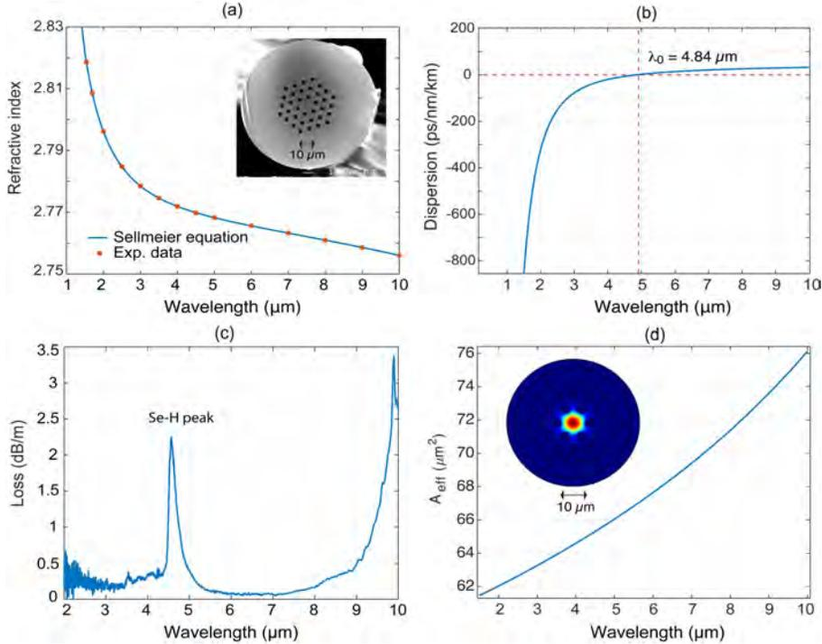
Figure 3: (a) Refractive index of  $\text{As}_{38}\text{Se}_{62}$  glass calculated with the Sellmeier model. Inset shows the cross-section image of the microstructured chalcogenide fiber. (b) Computed dispersion curve for the microstructured chalcogenide fiber with a zero dispersion wavelength near  $5 \mu\text{m}$ . (c) Absorption loss of the chalcogenide-based microstructured fiber. (d) Computed effective mode area. Inset shows the fundamental optical  $\text{HE}_{11}$  mode.
