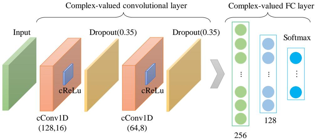
Fig. 5. Architecture of our proposed DC-CNN algorithm model.
