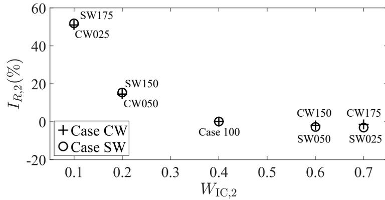
**Figure S5.** Improvement ratio ( $I_{R,2}$ ) in Case CW and Case SW as a function of the width of Inlet 2 ( $W_{IC,2}$ ).
