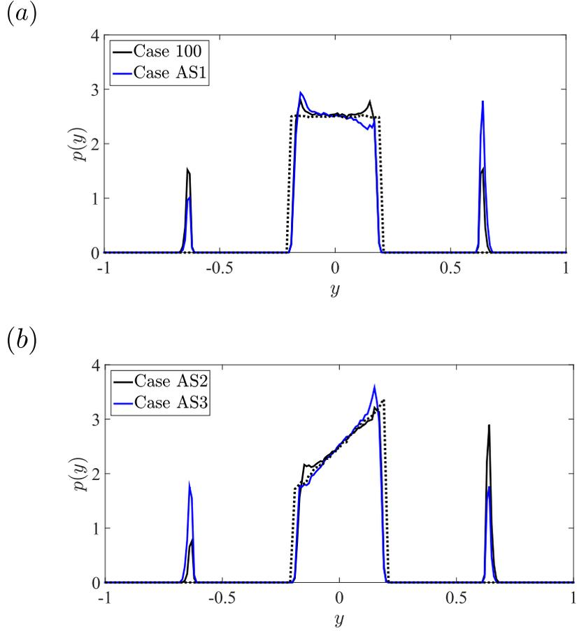
**Figure S13.** Probability density function of the particles at  $x = 163.84$  with an asymmetric initial distribution of particles given by Equation (S3). Dotted line shows the initial distribution of particles.
