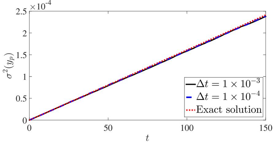
**Figure S3.** Time trace of  $\sigma^2(y_p)$  (i.e., the variance of  $y_p$ ) calculated using 200,000 Brownian particles injected from a point source in a uniform flow field.
