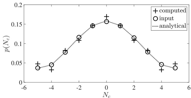
**Figure S16.** Charge distribution of particles computed from the number of particles classified by the PPPS in Case CD4 with significant figures of two digits.
