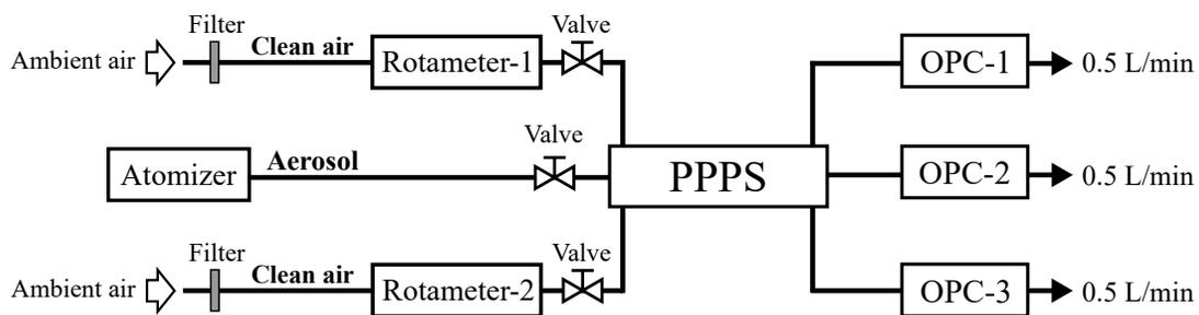
**Figure S2.** Schematic of the experimental setup.
