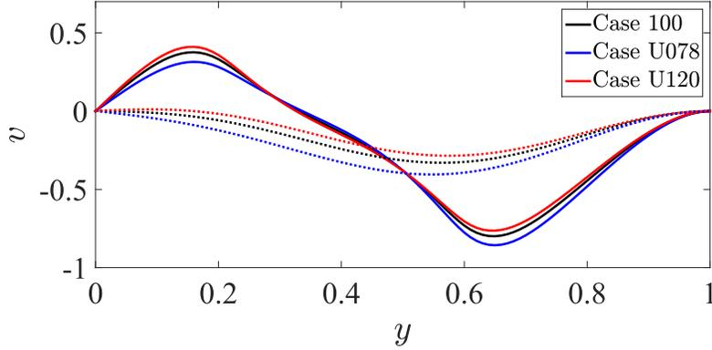
**Figure S7.** Wall-normal velocity of fluid  $v_f$  in Case U078, Case U120, and Case 100. Dotted line, at  $x = 10.12$ ; solid line, at  $x = 10.60$ .
