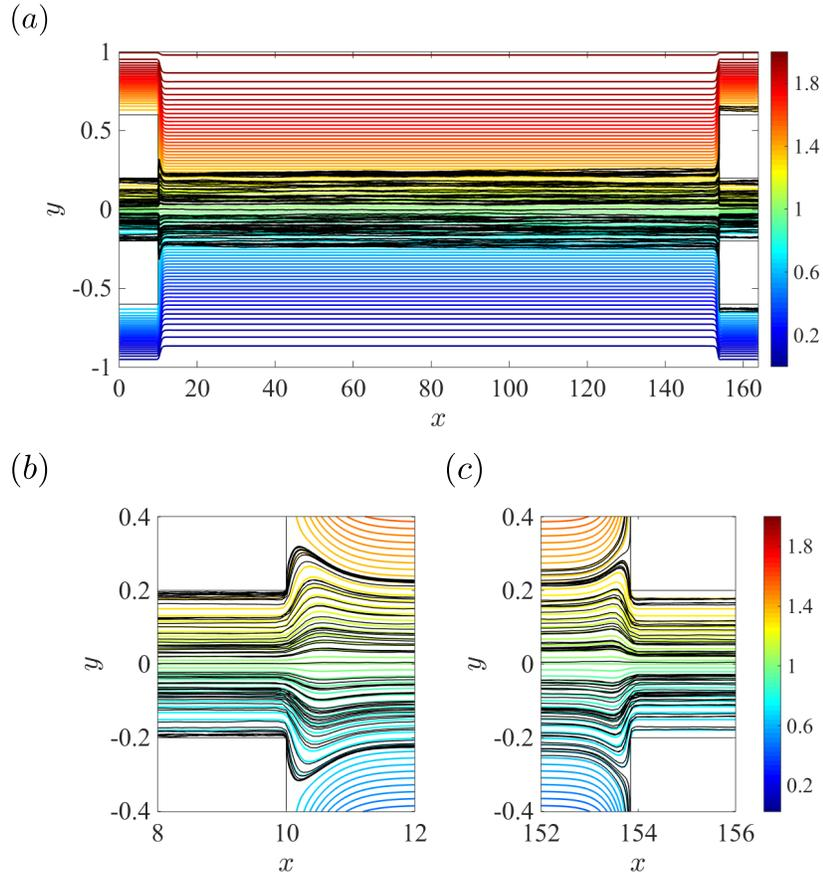
**Figure S4.** Streamlines and particle trajectories of 50 particles in Case 100: (a) overview; (b) upstream side of the classification section; (c) downstream side of the classification section. Colored line, streamlines; black line, particle trajectories.
