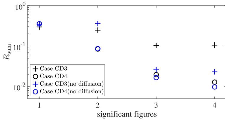
**Figure S15.** Sum of the residuals,  $R_{\text{sum}}$ , as a function of the significant figures for the computation of the charge distribution of particles.
