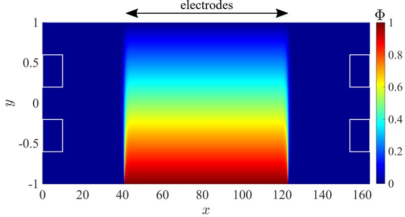
**Figure S9.** Distribution of the non-dimensional electric potential  $\Phi$ . the positive electrode is at  $40.96 \leq x \leq 122.88$ ,  $y = -1.00$ , and the negative electrode is at  $40.96 \leq x \leq 122.88$ ,  $y = 1.00$ .
