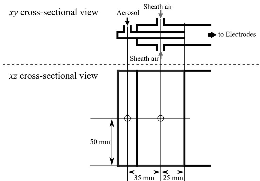
**Figure S1.** Schematic of the inlet section redrawn based on the figure of Okuda, Gunji, and Lenggoro (2015).
