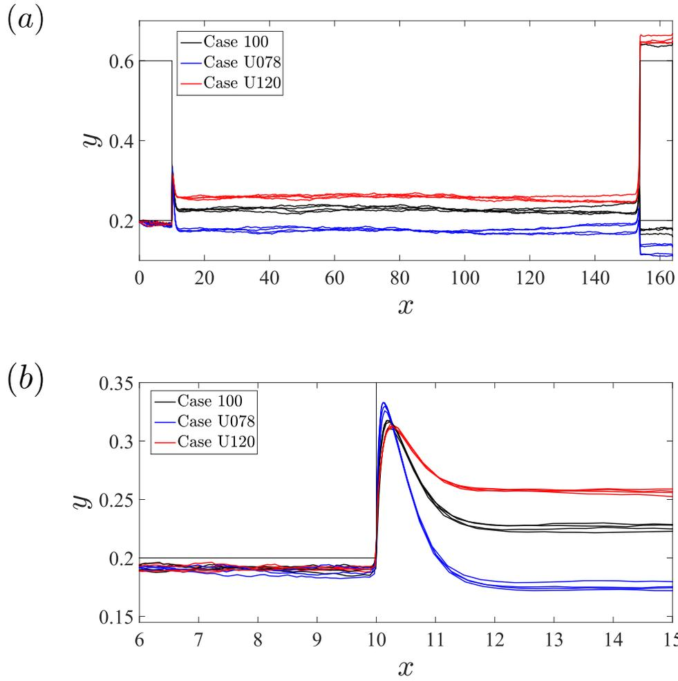
**Figure S6.** Sample trajectories of four particles close to the upper wall of Inlet 2: (a) overview; (b) zoom-up view of the upstream side of the classification section.
