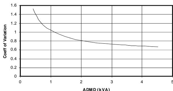
Fig.2: Relation between admd (expressed in kVA at nominal voltage) and coefficient of variation [2]
