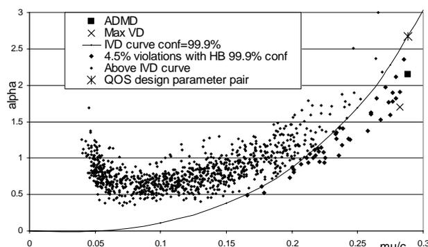
Fig. 3: BPP for Wn, 22-28 Jul 2000. (c=51.1A, n=65), using 10-minute data, with IVD curve for HB conf=99.9%, showing measured admd, and the load point with maximum voltage drop
