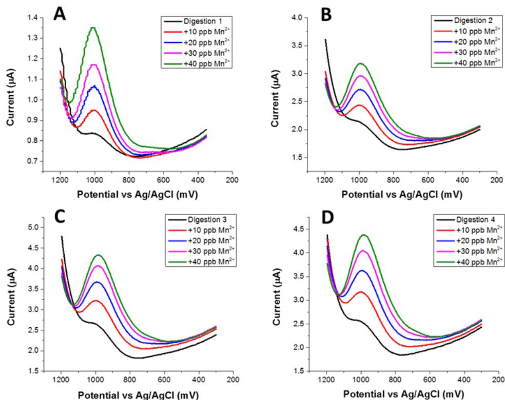
was from a fresh batch of Na-Heparin bovine whole blood. Deposition potential: +1200 mV; deposition time: 3 min
