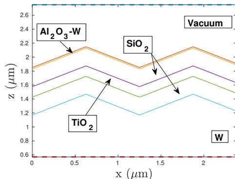
FIG. 4: Bragg-tungsten structure with sawtooth periodic interfaces.
