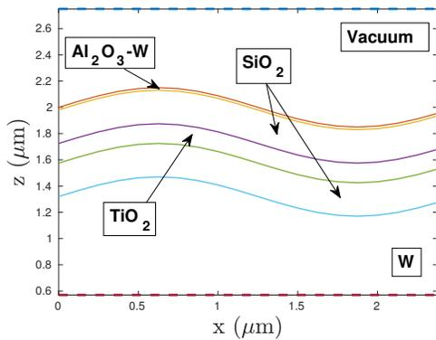
FIG. 2: Bragg-tungsten structure with sinusoidal periodic interfaces.
