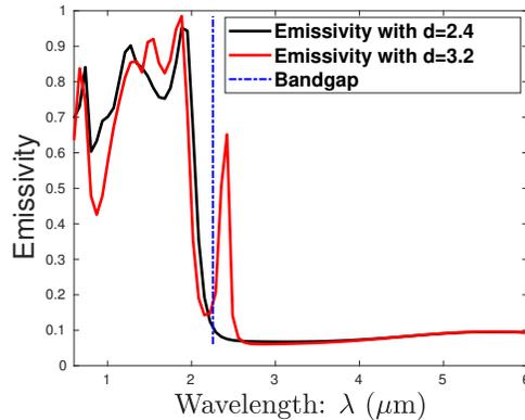
FIG. 7: Emissivity versus wavelength for periods  $d = 2.4 \mu m$  ( $d < 2\pi/\lambda_{BG}$ ) and  $d = 3.2 \mu m$  ( $d > 2\pi/\lambda_{BG}$ ) corrugated interfaces. ( $N_x = N_z = 20$  and  $N = 20$ .)
