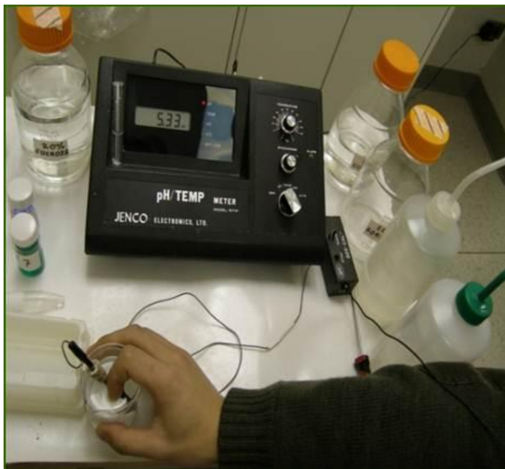
Figure 7. Creation of salt bridge in 3M KCL solution
