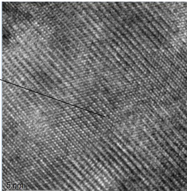
Figure 22. Grain boundary defect
