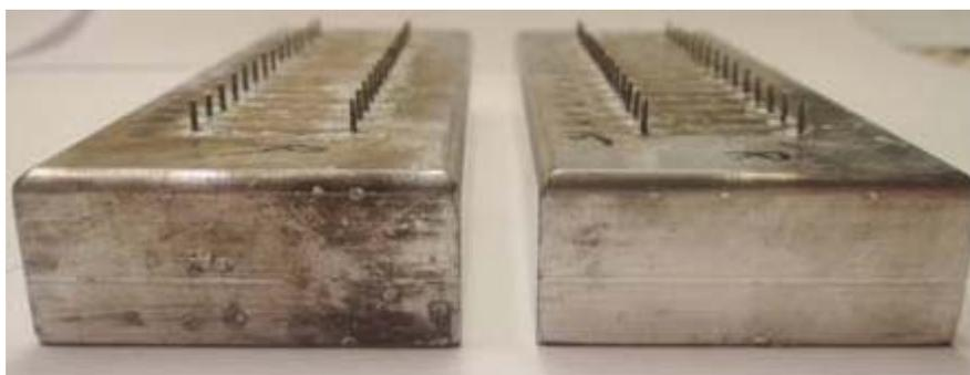
Figure 2. Aluminum blocks with 0.80 mm diameter pins set 19.05 mm apart.
