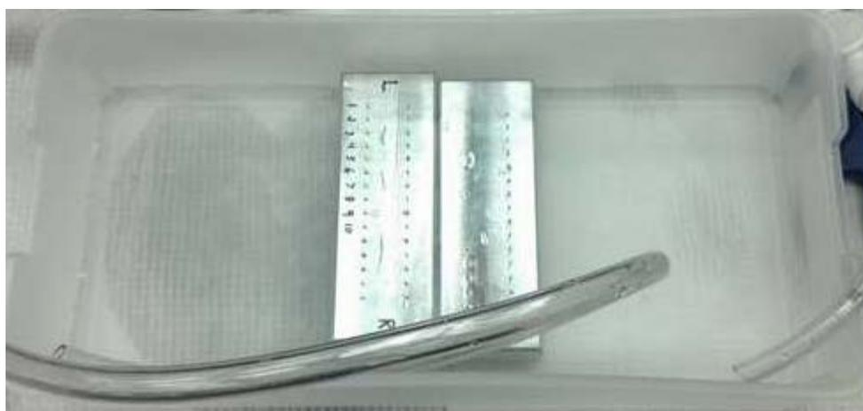
Figure 4. Water tank with two aluminum blocks submerged. The tubes are for water flow in and out.
