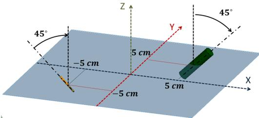
Fig. 2: Geometry for example. There are a thin PEC at (-5, -5) cm and a thicker dielectric cylinders at (5, 5) cm which intersect the  $xy$  plane at a  $45^\circ$  angle.
