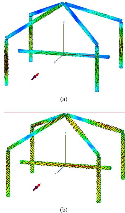
Fig. 1: Impressed currents on a geometrical structure made of (a) PEC and (b) dielectric material with  $\epsilon_r = 5$ . The polarization of the incident plane wave is indicated by the red arrow.
