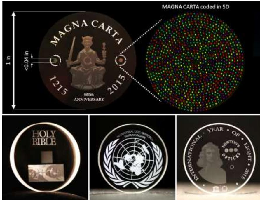
*Figure 2. These are photos from the University of Southampton that show one-inch discs that data is encoded to with micron-sized dots not to scale (Vincent, 2016).*
