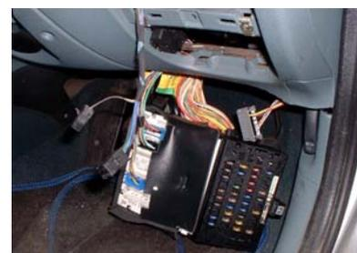
All the connections shown need to be made to connectors on the top (black) face of the unit.
