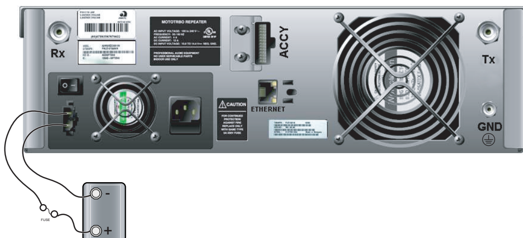
Figure 4-2 Making Connections to a Backup Battery
