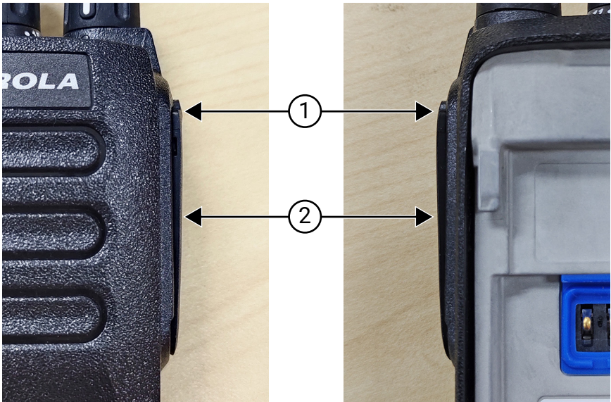
Figure 3: Dust Cover Not Secured
