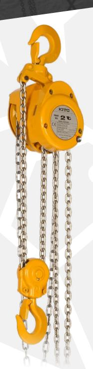
With a weight of just up to 28 kg KITO's CF model is ideal for its ease of handling and portability. The KITO CF is unique with its single reduction gearing that results in lifting speeds up to 28% faster than typical manual chain hoists. Moreover it is built with double pawl springs, and heavy duty heat-treated pinion and gears. The gear shafts with ball bearings minimize friction to guarantee ease of operation.
