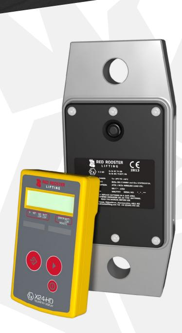
The RRI-T-ATEX load cells are manufactured from a high strength low weight Duralloy with a factor of safety of 7:1 on the smaller cells and 5:1 on the larger cells with all being proof loaded to 150% of the rated capacity.
