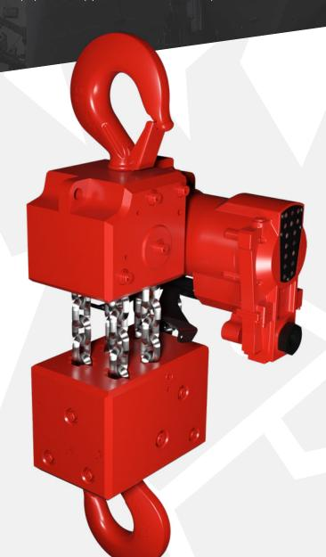
The new **Red Rooster Lifting** TMH series air hoists have the highest lifting speed with the lowest headroom on the hoist market. The TMH hoists are designed to operate at full lifting capacity with an air pressure from 4 – 6.3 bar. For full speed operation the hoist air pressure should be 6.3 bar.
