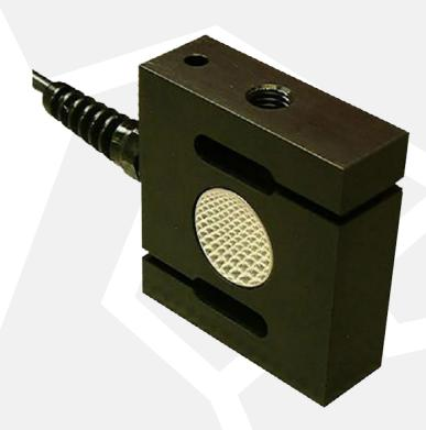
This compression load cell is manufactured in a range of capacities from 0.5 kN to 50 kN from high strength aluminium. It can be wired for tension or compression.
