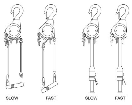
For the pendant control, adjust the speed by varying the amount the lever is depressed. By depressing the lever slightly, you will be able to control the hoists motions slowly with more precision. By depressing the lever further, the speed of the hoist will be increased until the lever is fully depressed.
