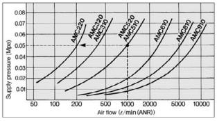
How to view the diagram: If the AMC510 is operated at a flow volume of 1000  $\ell$ min (ANR), the supply pressure will be 0.05MPa.
