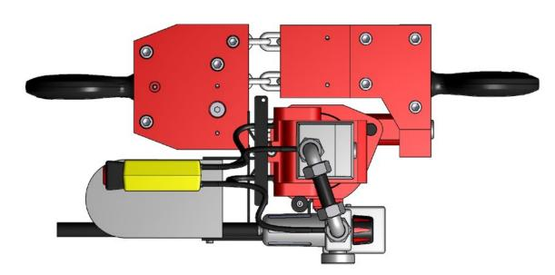
Air Hose Connection with Hose Clamp and Manifold
