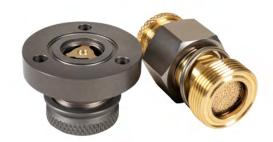
Danfoss Hansen LF series is a specific coupling made for industrial applications using SF6 gas. Its design allows a perfect sealing over several decades and an extremely limited permeation of media into the atmosphere during connection and disconnection, in order to limit global warming. The coupling has a dual O-ring design and dust caps ensuring tight sealing while it is disconnected
