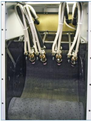
For saturation treatment of small components in bulk which are gently tumbled at constant speed under an air powered blast stream on a perforated endless belt made in abrasion resistant rubber. The EBI can be used with hard, fast cutting abrasives such as aluminium oxide, 'soft plastic' media or low density glass bead.
