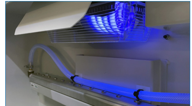
Above: The Formula 1400 CCR blast cabinet is fitted with ultra-violet lighting. Some conformal coatings, that are UV cured, give an enhanced fluorescent response which makes the coating more visible under these 'black lights' so aids operator accuracy when blasting
