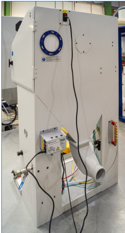
Left: Rear of Formula 1400 CCR cabinet showing ionised air power box, busbar for earthing, quick release breather pad filter
