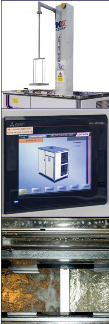
The Kerry Microsolve Mono-Solvent system manufactured by Guyson has three process stages comprising of ultrasonic cleaning, followed by vapour rinsing and freeboard drying. The Microsolve has unique proven solvent retention features that provide economic benefits as well as effective use of HFE (hydrofluoroether) or HFC (hydrofluorocarbon) solvents.
