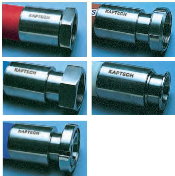
To comply with FDA requirements, all hose liners are manufactured from 316 stainless steel. Hose ferrules and nuts (where applicable) are manufactured from 304 stainless steel.
