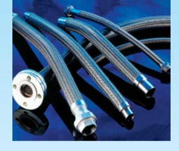
**Design & Installation:** Kaptech Stainless Steel flexibles should be configured and installed in such a way that the minimum bend radius is not exceeded, the hose is not stretched, compressed nor twisted, and the external braid is not subject to wear nor damage.
