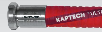
Its structure of synthetic fabric plies and embedded high tensile wire helix gives exceptional vacuum and pressure performance. The convoluted outer surface optimizes flexibility and ease of handling.
