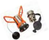
Dry Gas Couplings are a further development from the DDCouplings specially designed to handle LPG (Liquified Petroleum Gas) even during the toughest conditions. DGCouplings are available in sizes from 1" to 8" and various types of connections to handle almost any type of LPG transferring. According to standard EN 13760:2003(E).
