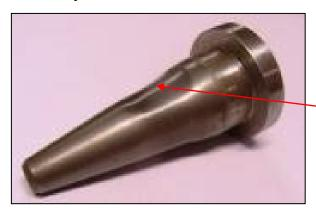
The airjet should be withdrawn from the gun body after 8 hours blasting to establish the wear pattern on its outer surface. When wear has become noticeable, the fitting should be rotated to the next unworn section. When wear has occurred around the whole circumference, the airjet should be replaced.
