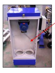
Carefully remove filter from dust collector.
