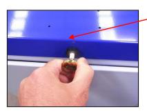
Shake filters and allow dust to settle
