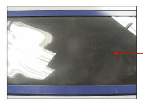
Check that the view of the component to be air washed is not impaired by a dirty anti frost sheet (P2PF0008 or P2PF0005 for the Formula 1200) or glass (P2GL0008 or P2GL0001 for the Formula 1200). Replace if necessary.
