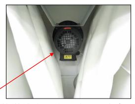
On a F41 dust collector the motor is inside. Unclip the catches and remove the front panel to check its rotation.
