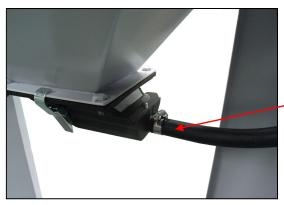
Check the media supply hoses (R6TB0018 for F1400 and F1600, R6TB0014 for F1200) for signs of wear and damage. Internal wear can be determined by feeling the rigidity of the tubing along its length. Any internal wear will result in the hose feeling soft where the hose wall is thinner. The first section to go is usually next to the pickup tube.
