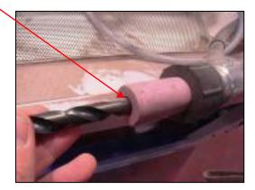
The picture below shows an extremely worn nozzle. Your nozzle should reach this state as it will decrease its blasting effectiveness and may also damage the blast gun.
