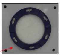
Remove and replace the breather pad **(Y1AB0001)**. Return the breather bezel to the locked position.
