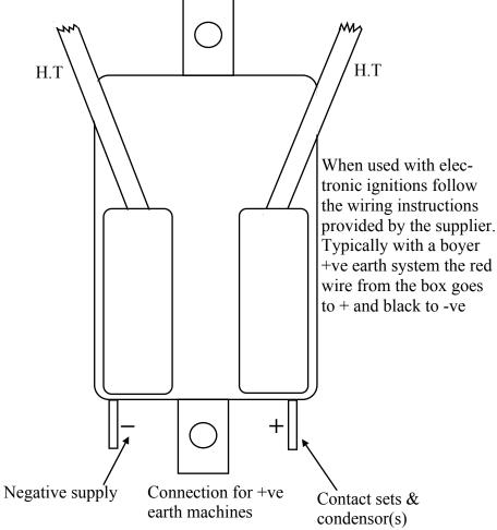
For -ve earth systems, contact sets and condensor(s) go to -DC positive to +
