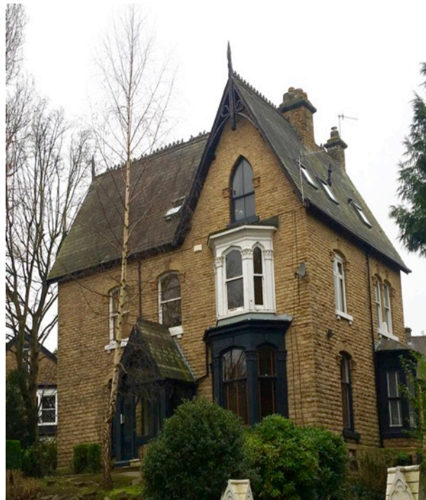
Again the gothic references in these two houses can be seen in the pointed arches above the windows and the steep roof.
