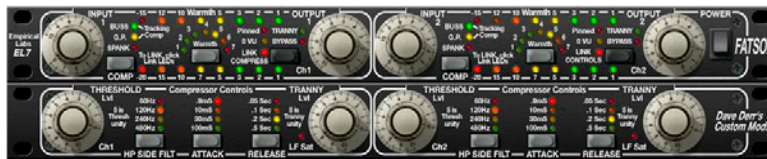
Figure A10.14 Empirical Labs EL7 FATSO recreates the warm, musical qualities of magnetic recording tape, tubes, and class A transformers.
