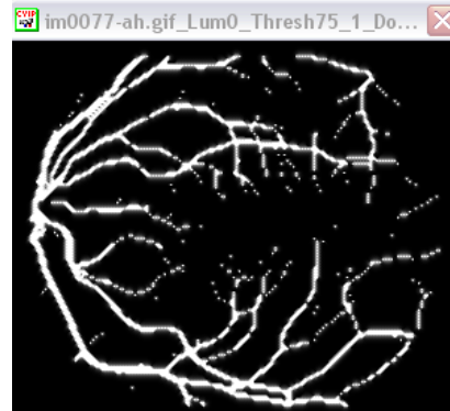
Fig 23: Binary-converted hand drawn image from the STARE database. It was first converted to gray scale, then binary thresholded at a gray-scale value of 75.
