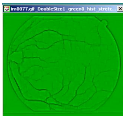
Fig 9. A 2 nd morphological filtering operation. An opening operation using a size-15 rectangular structuring element split objects that were connected by narrow strips and eliminated peninsulas from the edge detected image.
