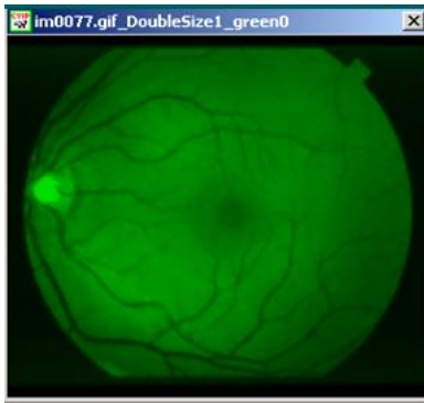
Fig 5. Preprocessing step 1. Extraction of the green band from the resized, original, color image helped enhance image details.
