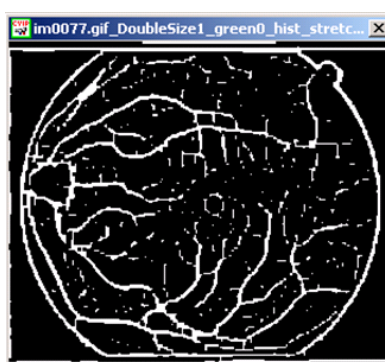
Fig 12. Post processing step 3: Logical NOT operation & Hough Transform. The NOT operation produced a black background. The Hough transform was used to attempt reintegration of bifurcation points and vascular branches
