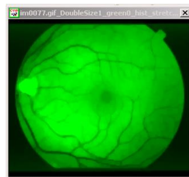
Fig 7. Morphological filtering operation. An opening operation with a size-5 rectangular structuring element smoothed the vessels' geometries.
