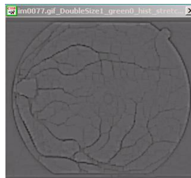
Fig 10. Post processing step 1: Color-to-gray-scale conversion. This is the result of the intermediate step of converting the color image to a binary
