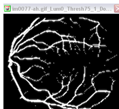
Fig 13. Ophthalmologist's hand-drawn image converted to a binary image for comparison to algorithms' output images.
