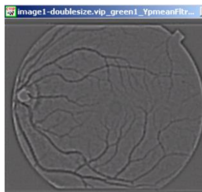
Fig 20. Algorithm 2: Post processing step 2. Color-to-gray-scale conversion is the intermediate step to converting the color image to a binary image.
