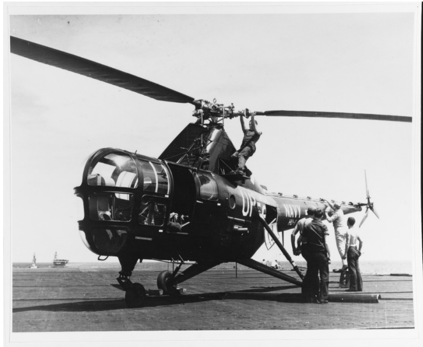
A Sikorski HO3S-1 helicopter on board the USS Philippine Sea (CV-47) during operations off Korea, October 19, 1950. The crewman is backing off vacuum prior to starting the helicopter's engine.
