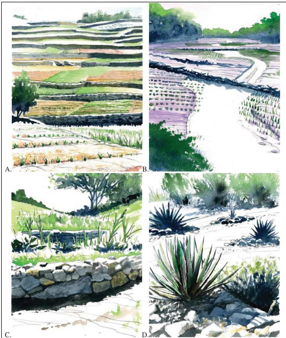
FIGURE 11.3 Sketches of the four types of surface runoff control we describe in this chapter including (A) linear alignments, (B) water spreaders, (C) channel terraces, and (D) rock mulches. Illustrations by Caldwell Design.
