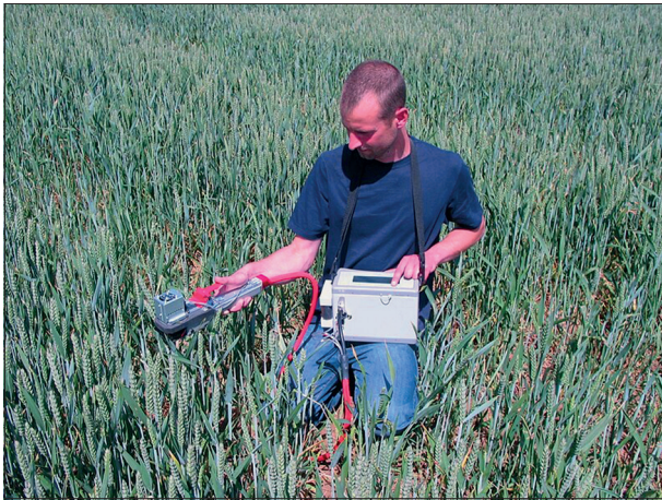
Figure OM4.5-2 A portable IRGA in use in a wheat field. The researcher is supporting a box containing a computer, gas supplies, and batteries. The silver box on the hand-held device is the leaf chamber, clamped onto a wheat leaf. (From "Measuring photosynthetic efficiency using an LCpro-SD," by Steveaducuk, Wikimedia.)
