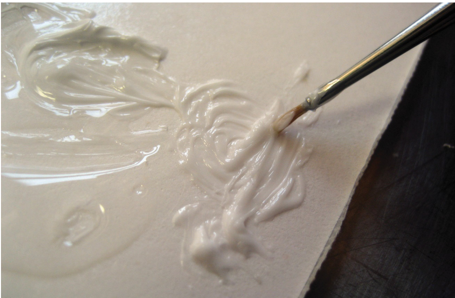
FIG. 10.21 Mixing thickened silicone Image reproduced by permission of Maddie Singer
