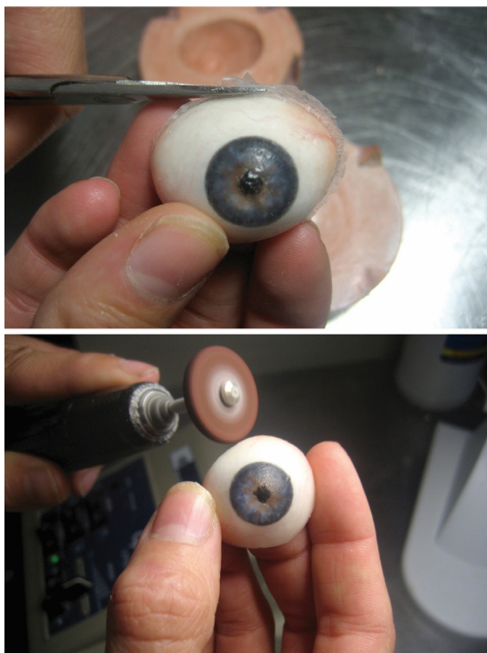
FIG. 10.28 Trimming de-molded eye (top); Grinding edge (bottom)
