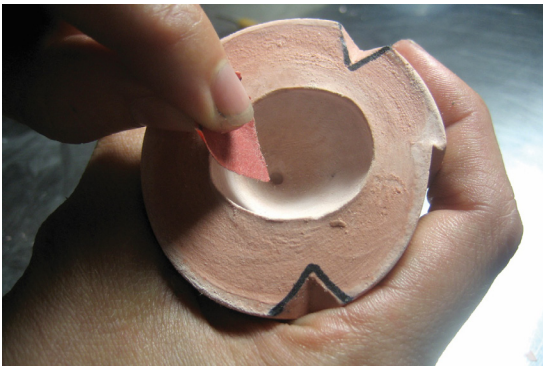
FIG. 10.08 Sanding prior to coring Image reproduced by permission of Maddie Singer
