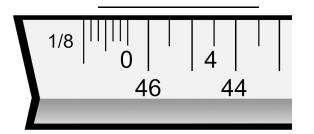
TO DETERMINE THE NUMBER OF INCHES, SIMPLY SLIDE THE SCALE RULE SO THAT THE LINE ENDS AT THE 6' MARK AND THEN COUNT BACKWARDS THE NUMBER OF INCHES IN THE INCH SCALE.
