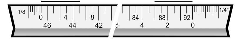
EACH OF THE TICKS FOLLOWING THE ZERO REPRESENT A MEASUREMENT OF FEET.
