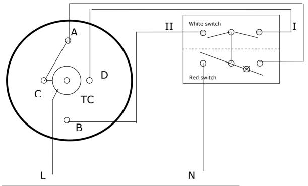
Looking down into the machine at switch with element on left hand side of the switch
