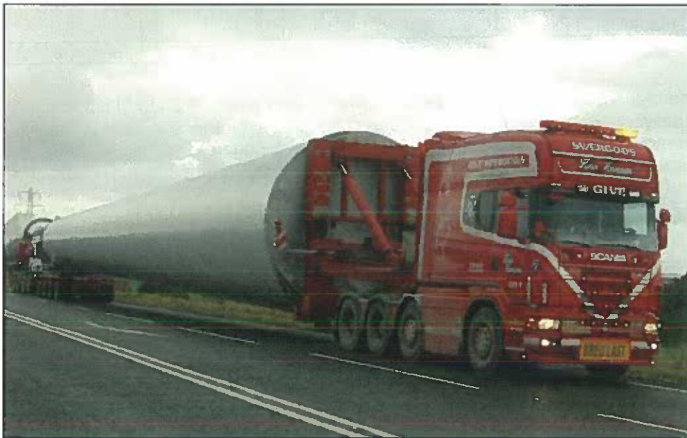
Photograph 12.3 Typical tower transport
