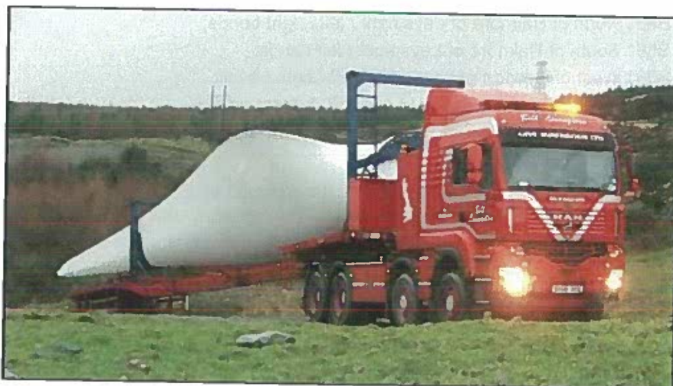
Photograph 12.1 Typical blade transports
