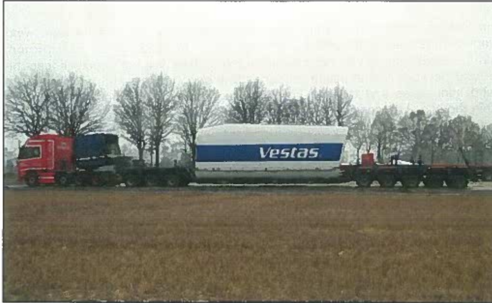
Photograph 12.2 Typical nacelle transport
