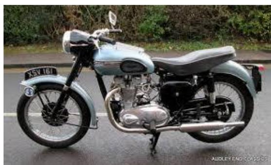
With the sales success of the Triumph Speed Twin, Edward Turner, Triumph's motorcycle designer, looked further into developing the potential of the new parallel twin motor. The lighter and more powerful Tiger 100 was developed as a sports enthusiasts' machine, and as with previous models the "100" referred to its claimed maximum speed in miles per hour (mph).
