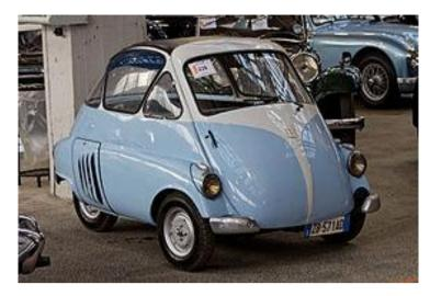
The car originated with the Italian firm of Iso SpA. In the early 1950s the company was building refrigerators, motor scooters and small three-wheeled trucks. Iso's owner, Renzo Rivolta, decided to build a small car for mass distribution. By 1952 the engineers Ermenegildo Preti and Pierluigi Raggi had designed a small car that used the motorcycle engine of the Iso Moto 200 and named it Isetta.
