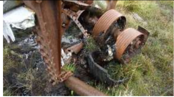
Pl 13. Wheel gear with last remnant of tyre surviving.
