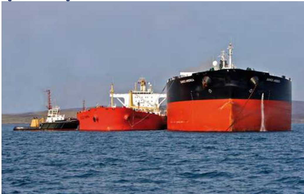
Figure 4-1: STS cargo transfer
