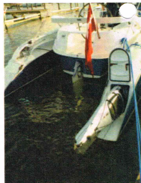
One or two kayakers, a small catamaran which can be dismantled... The volume in the floats acts as a spacious luggage carrier...
