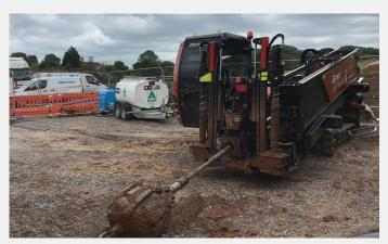
HDD machine for drilling under roads and rivers
