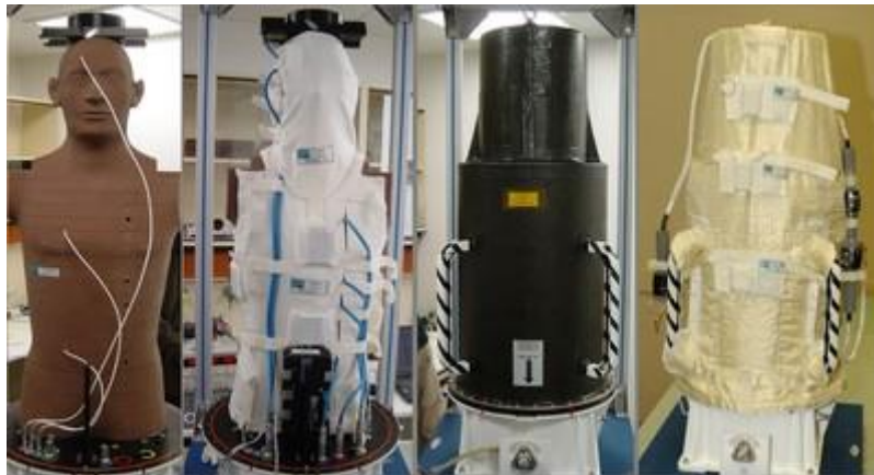
During the exposure in the open space, the MATROSHKA phantom was covered by a container imitating the shielding properties of a spacesuit. (Source: DLR)
